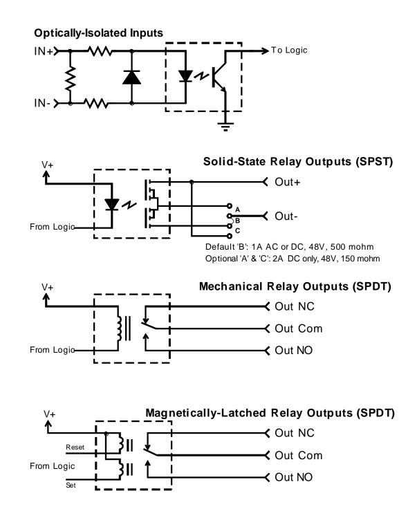
Figure 3 - I/O Equivalent Circuits
