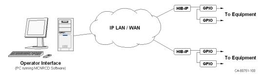
Figure 2 – GPIO in an MCN System
